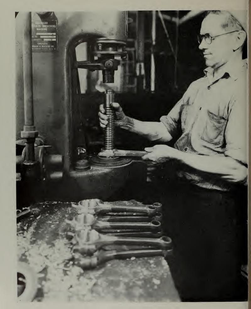
All babbitt bearings except the twenty per cent which are finished to special undersize on the lathe shown in Picture 22 are now finished to size by a hydraulicly operated broaching machine as shown in the above picture. The broaching tool which is used for this operation is held in the workman's right hand. It is composed of a number of horizontal cutters each of which removes about .0005 as the tool is forced through the bearing by the hydraulic pressure.
